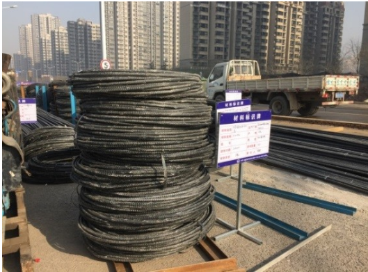
Figure 4 GFRP Stirrups of Piles
