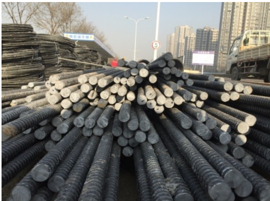
Figure 5 GFRP Reinforcements of Piles
