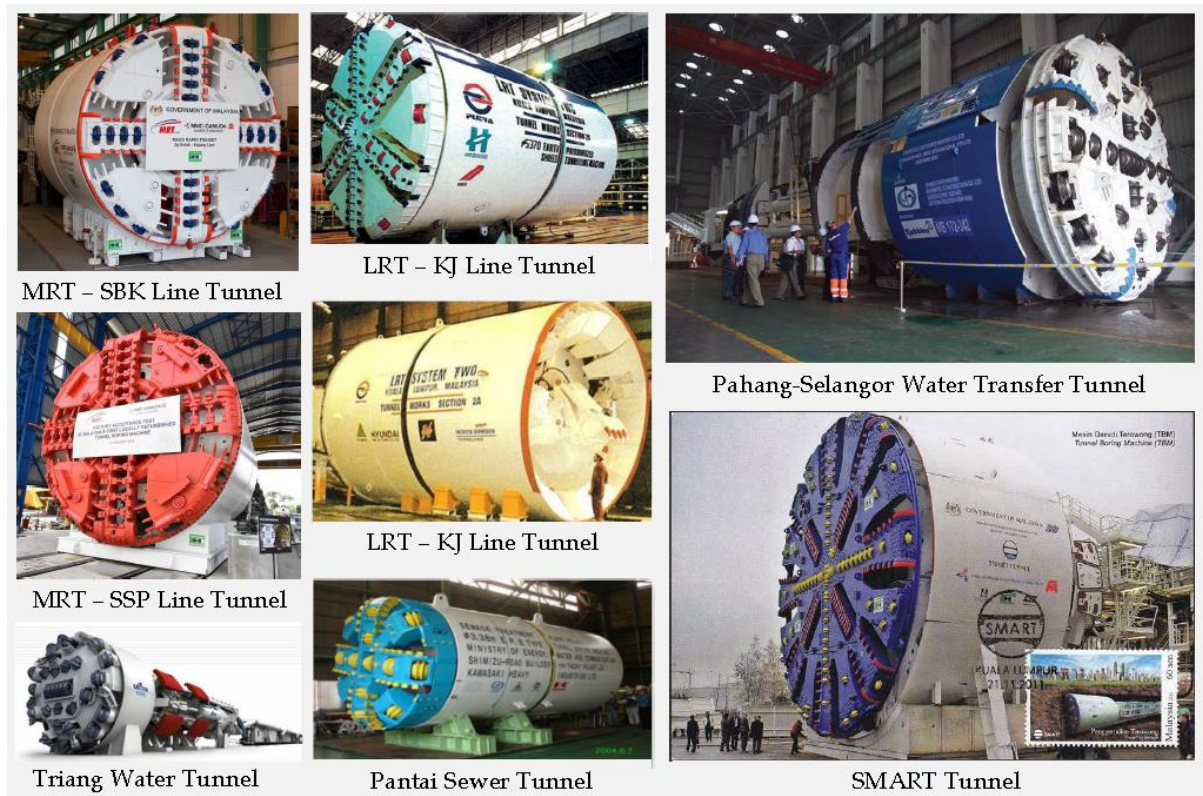
Figure 6: TBMs employed in past tunnelling projects
