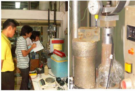
Figure 24 Suction-monitored unconfined compression test as an illuminating lab demonstration for MEng students at Kasetsart University
