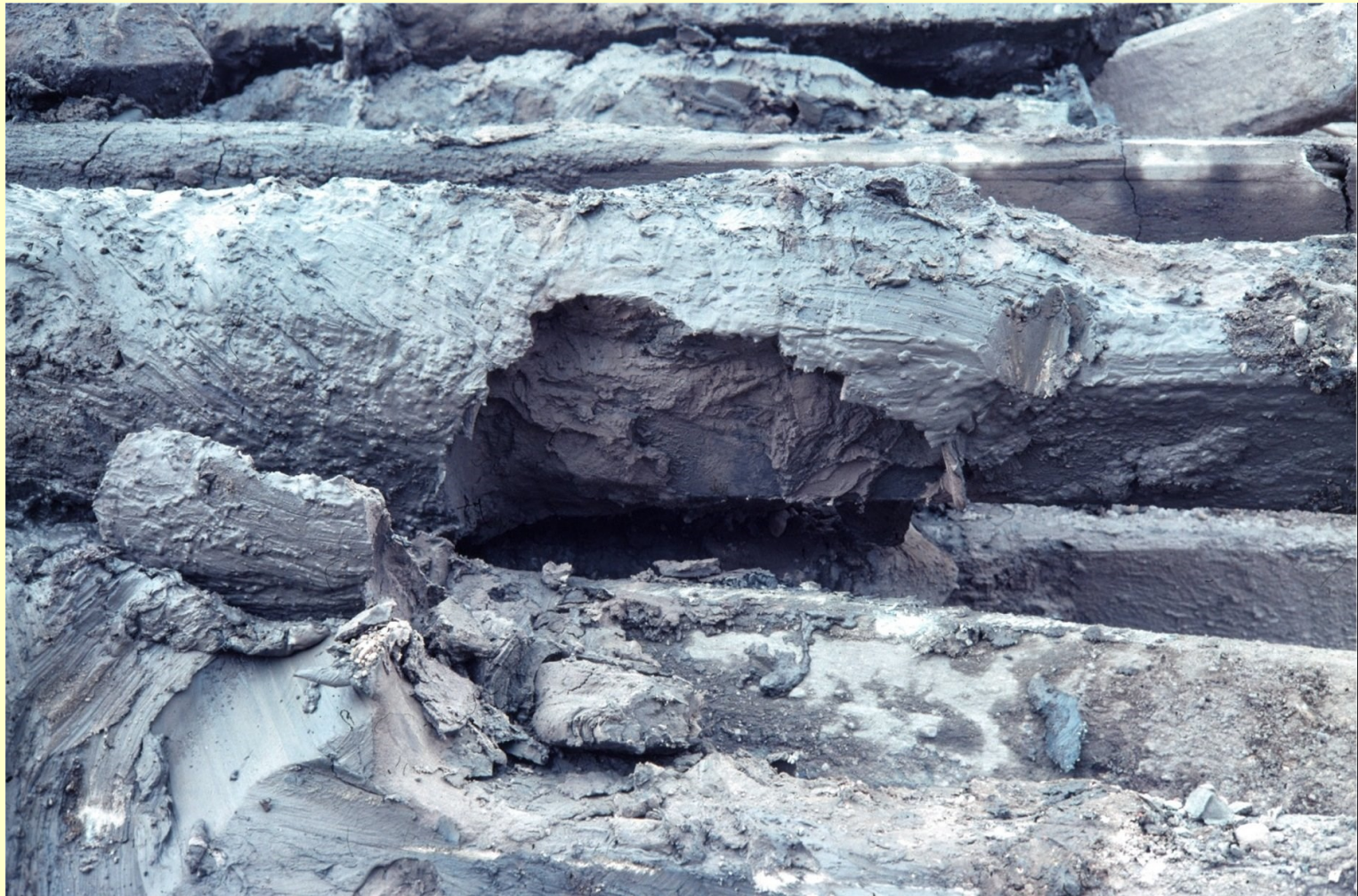
Clay adhering to extracted piles
