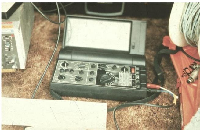
Figure 1 Vibration monitoring of resonance compaction in 1988, at Annacis Island, Canada, (Massarsch and Fellenius 2017)
