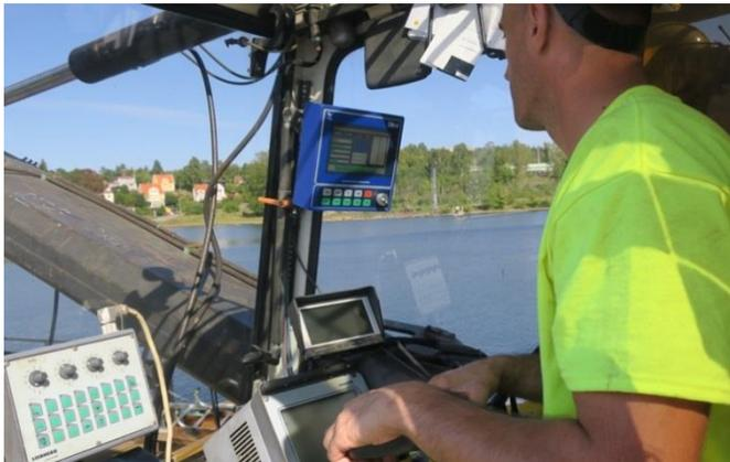
a) View of machine operator following driving instructions on MPCS screen
