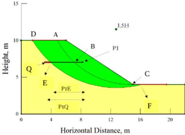
Figure 4 Critical slip circle for slope with  $Z_0 = 3.0$  m,  $L_r = 5.08$  m and  $FS_{min} = 1.51$
