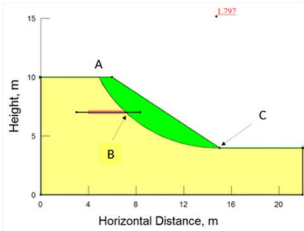
Figure 5 Reinforced slope with  $Z_0 = 3.0$  m,  $L_r = 5.08$  m analysed for failure slip circle ABC of unreinforced slope.
