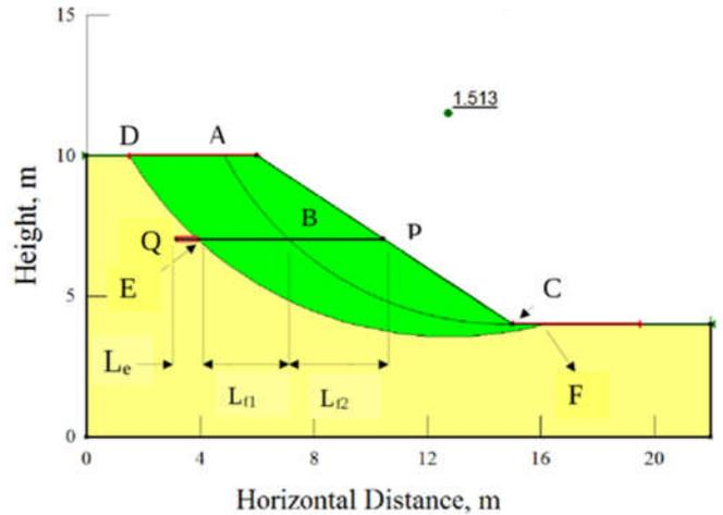
Figure 3 Critical slip circle for Z<sub>0</sub>=3.0 m, FS<sub>min</sub> = 1.51, L<sub>r</sub> = 7.27 m
