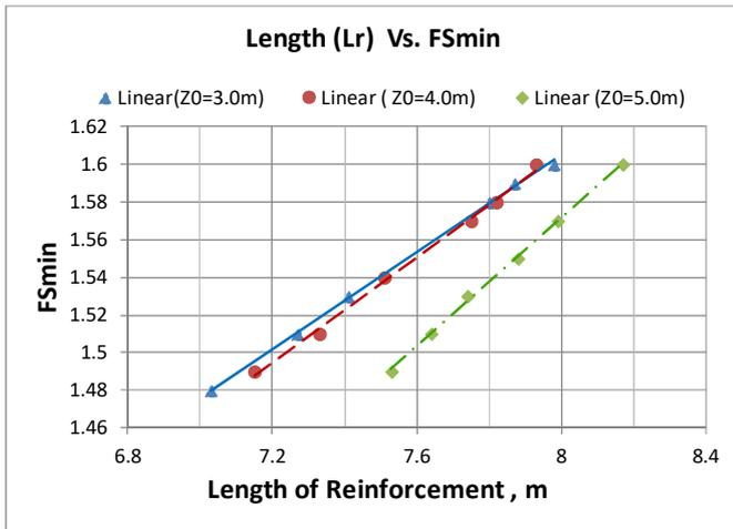
Figure 7  $FS_{min}$  vs.  $L_r$  for  $Z_0 = 3.0$  m, 4.0 m and 5.0 m
