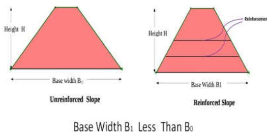
Figure 1 Comparison of Base Width Requirement for Unreinforced and Reinforced slope
