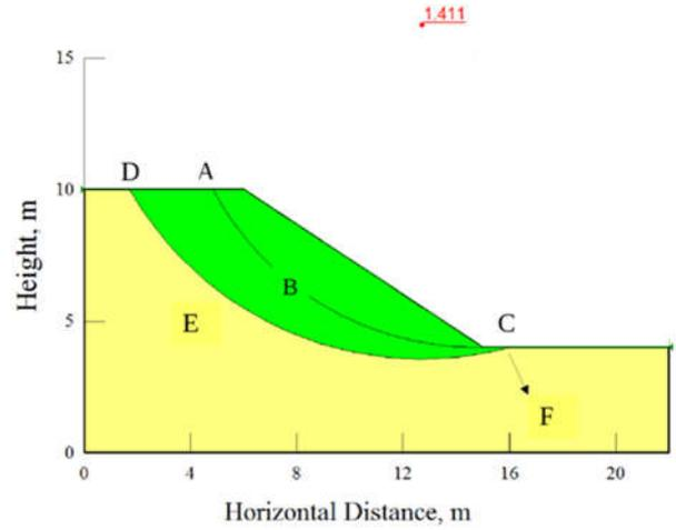
Figure 6 Slope stability with critical slip circle DEF but without considering the effect of reinforcement
