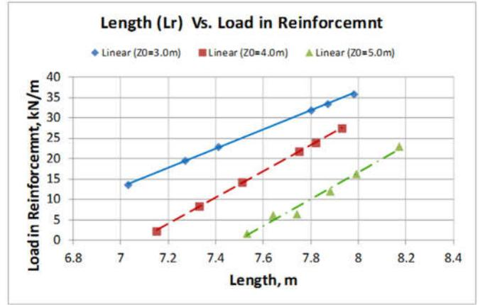
Figure 8 Load in Reinforcement,  $F_r$  vs. Length of Reinforcement,  $L_r$  for  $Z_0 = 3.0$  m, 4.0 m and 5.0 m
