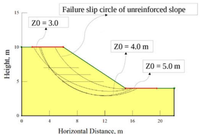
Figure 9 Critical slip circles for reinforcement at  $Z_0 = 3.0$  m, 4.0 m and 5.0 m and for unreinforced case
