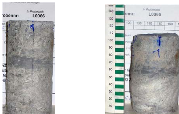
Figure 5 Kakirite specimen before and after CD-test
