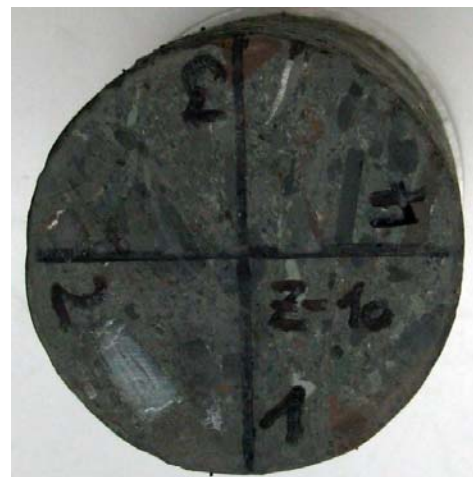
Figure 10 Section of a breccia specimen from the Gibraltar strait with visible hard inclusions
