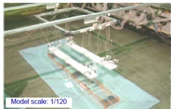
Fig. 3-4 Immersion operation vessel and hydraulic model tests to confirm the immersion procedures (Taisei Technology Center)
