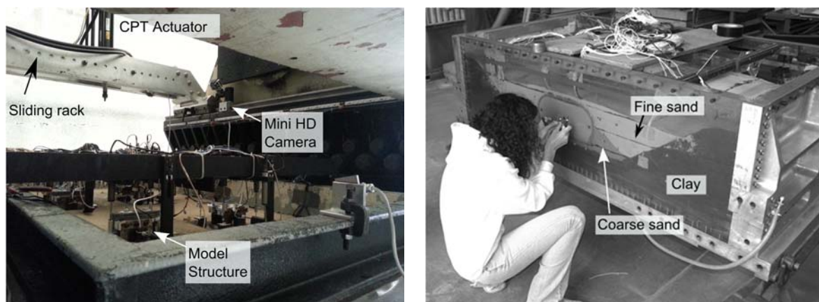
Figure 1: Centrifuge models of structure-soil-structure interaction problems with liquefying soil. (a) Several structures on shallow footings. High resolution and high speed cameras are used to monitor the structures while 150 sensors measure the model response. A servo-hydraulic actuator is used to drive a cone penetration test in flight. (b) Submerged transit tube with liquefying backfill. Dense pore pressure arrays define transient seepage patterns and non-contacting electro-magnetic position sensors track tube displacements. (Wilson and Allmond 2014)
