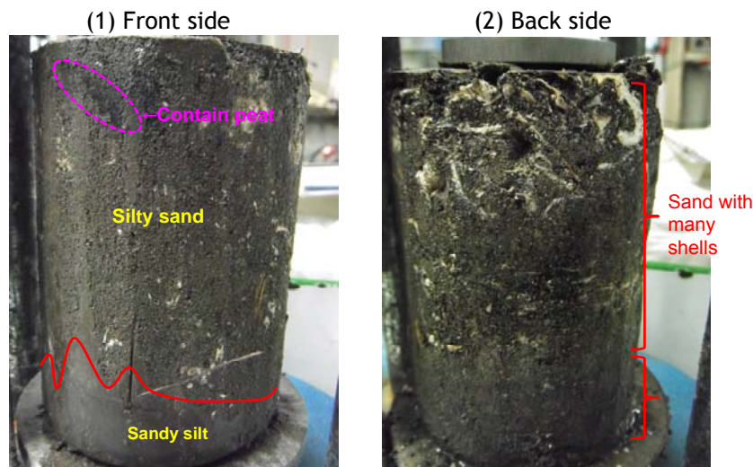
Photo 1 Non-uniformity of dredged and filled soil
