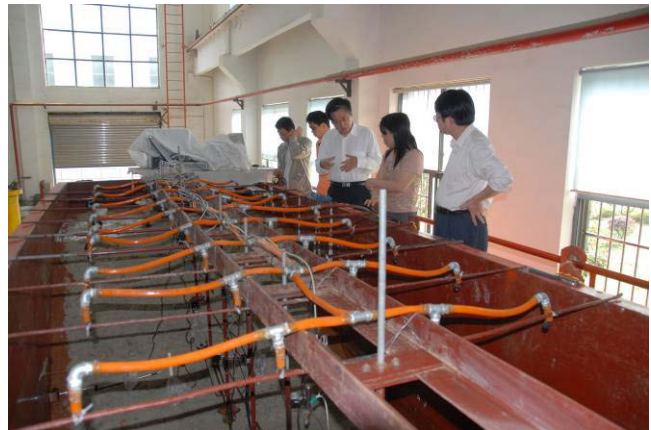
Figure 18 Prof. Z.L. Cheng explains an expansive soil model slope tested at 1g (with courtesy of Prof. B.W. Gong)
