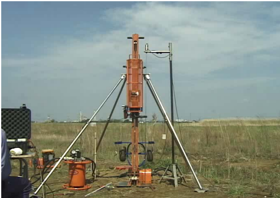
Fig. 3 Onshore practice of dynamic cone penetration.
