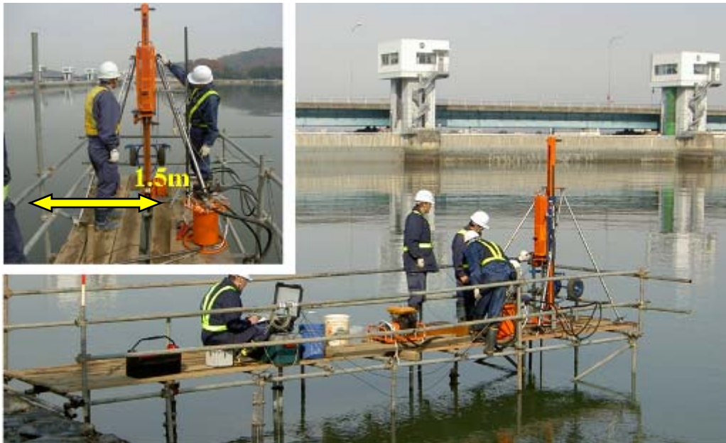
Fig. 5 Cone penetration test upon a small platform in river.
