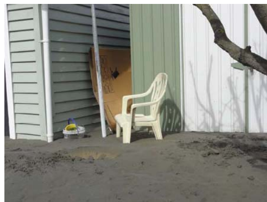
Figure 6. Evidence of extensive liquefaction (large sand boils) in residential areas of Avonside. Notice the chair embedded in 20 cm thick sand ejecta in the backyard of the property.
