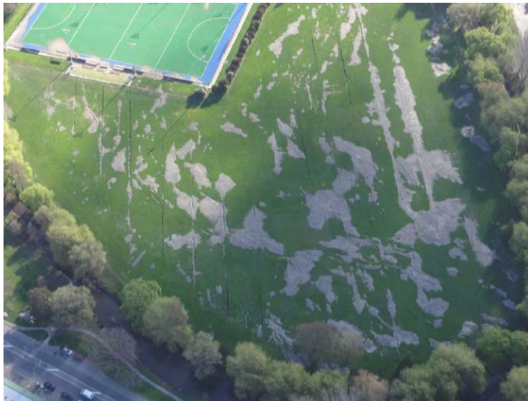
Figure 5. Evidence of extensive liquefaction (large sand boils) in Porritt Park, Christchurch. Using the vehicles (bottom of photo) or the hockey field (top of photo) for scale gives a good indication of the significant volume of sand ejecta.
