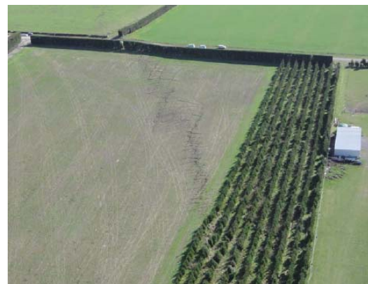
Figure 2. Surface fault rupture on farm land. The right lateral offset was approximately 4 m at the tree line (top of the photo)
