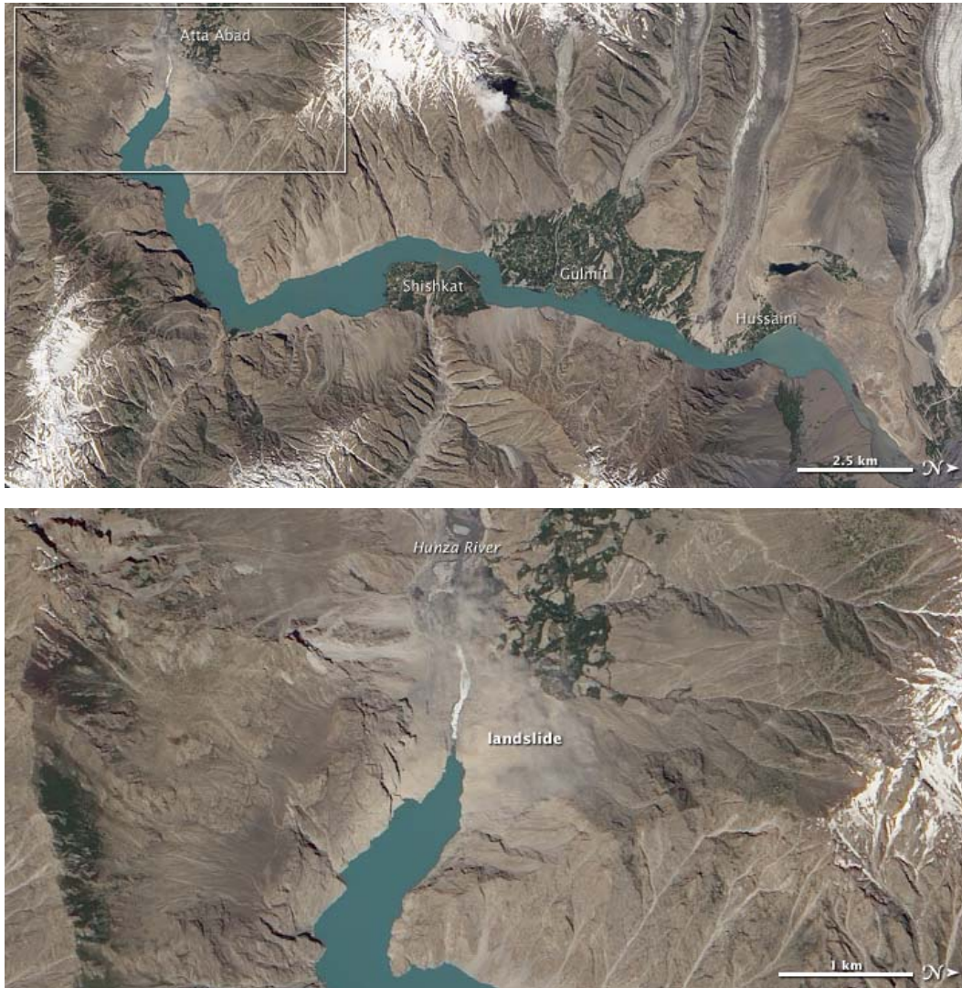
Figure 11 Image of over spilling Attabad landslide dam on July 7, 2010
