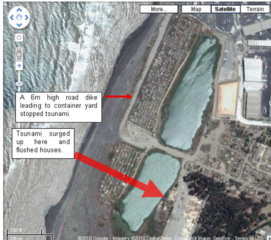
Photo 27 Tsunami protection by embankment (drawn on Google Map)
