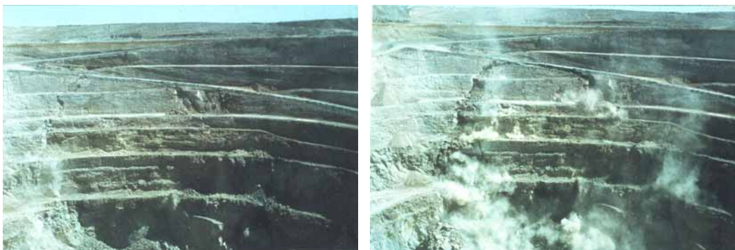
Figure 3. Large wedge failure in the Teutonic Bore open-pit mine in Western Australia caused by the presence of two pre-existing major fractures.
