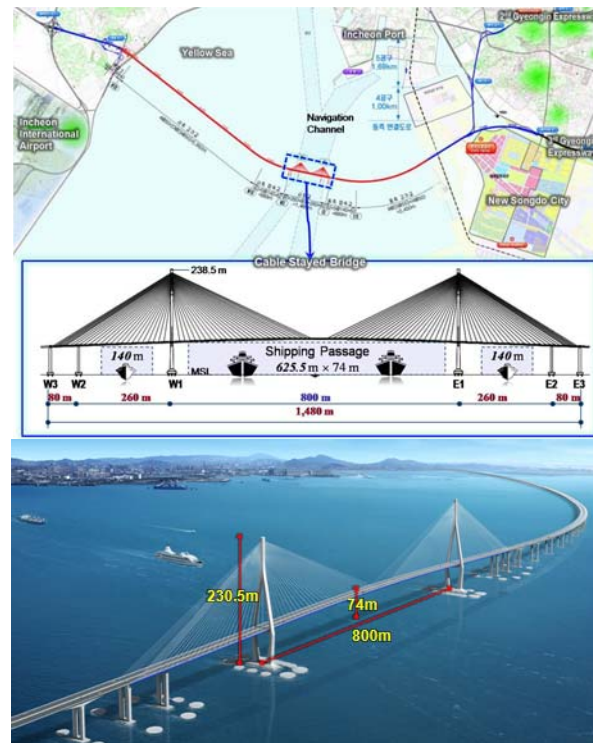
Figure 2. Route map of the Incheon Bridge and the cable stayed portion as its main section
