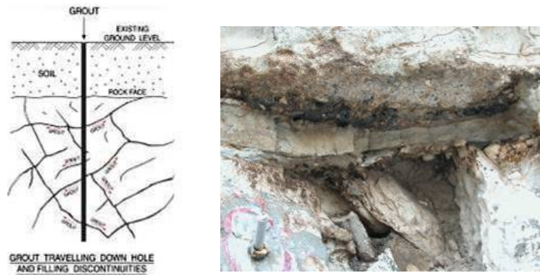
Fig. 8 Depiction of fissure grouting and end product
